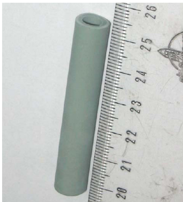
Fig. 8. Photograph of green body of NiO/YSZ anode tube made by gelcasting.
